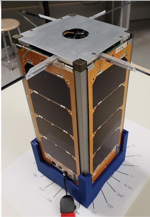
Cubesats are a type of small satellite with standardized dimensions. RamSat is a “2U” cubesat, with dimensions of 20 cm x 10 cm x 10 cm. It includes several component systems which work together to carry out its mission. RamSat’s solar panels provide power to charge a lithium-ion battery, which in turn powers a flight computer, cameras, navigational components, and a UHF/VHF radio for 2-way communication with a ground station in the Robertsville Middle School STEM classroom.
