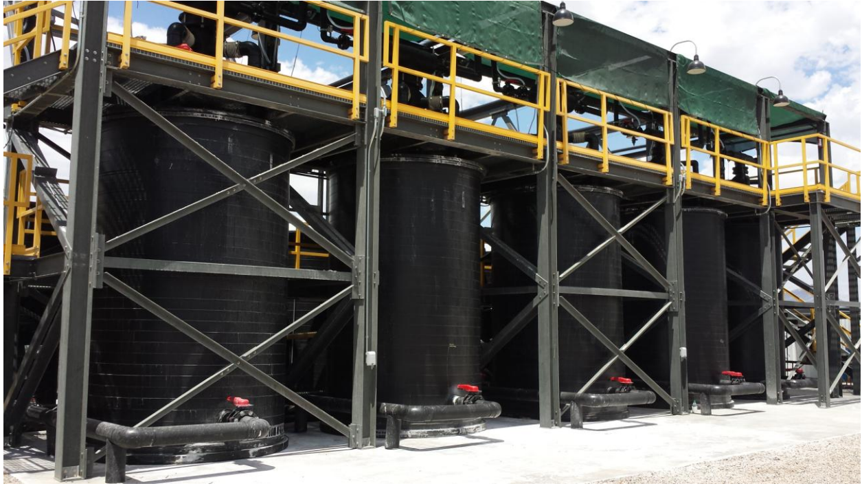
RAE's patented, high-volume algae harvesting system.
